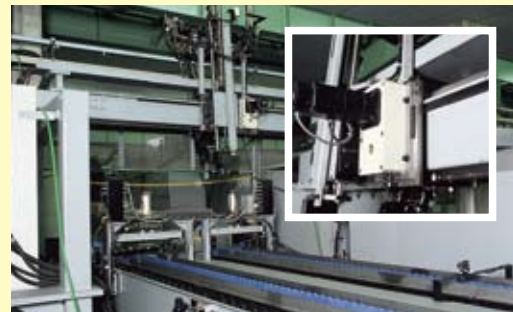
Automatic material handling equipment (CP racks &amp; pinions)
